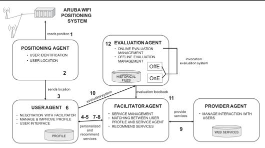
Figure 1 Schema of the multi-agent architecture.
