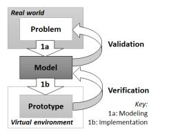
Fig. 2. The role of validation and verification in the prototype development.
