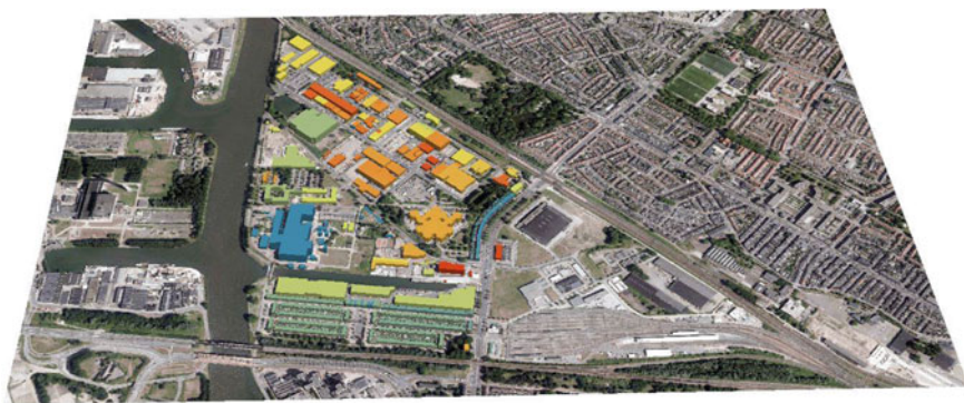
Fig. 129.5 Collecting and comparing data of buildings being (partly) demolished thus supplying materials (‘donor buildings’) and buildings in need for materials (‘receptor buildings’) (Jochemsen 2016)
