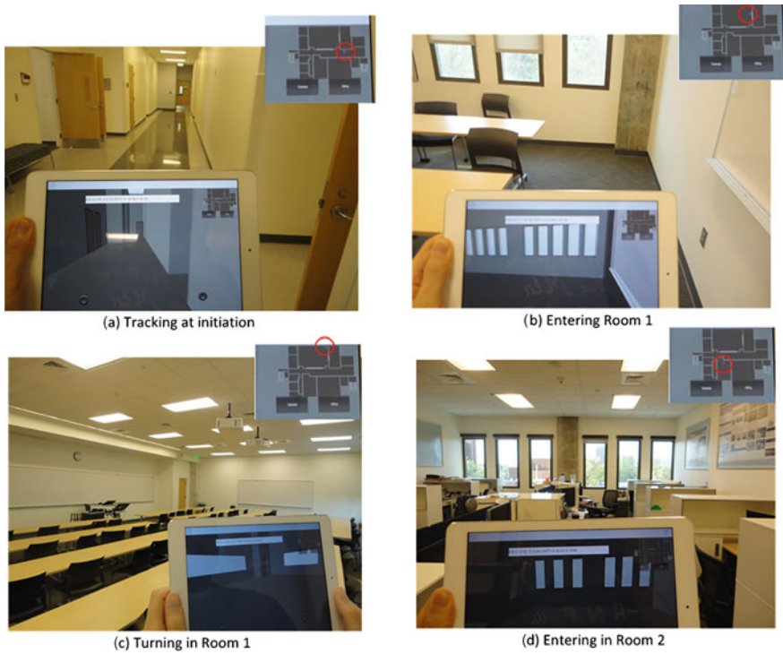
Fig. 135.7 Tracking test result and virtual BIM view
