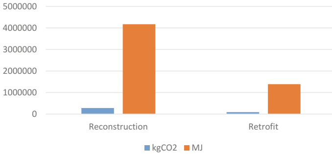
Fig. 28.6 Evaluation of environmental impact of rebar
