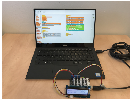
Fig. 7. Exemplary weather station project using a combined temperature and pressure sensor as well as a LCD attached to a grove shield.
