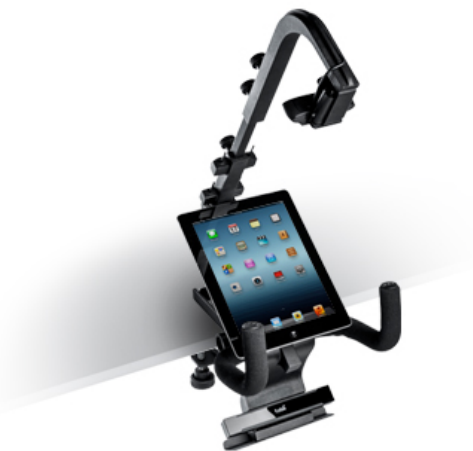
Fig. 3 Eye-tracker is placed on the bottom part of the stand, and the iPad is attached in the centre.
