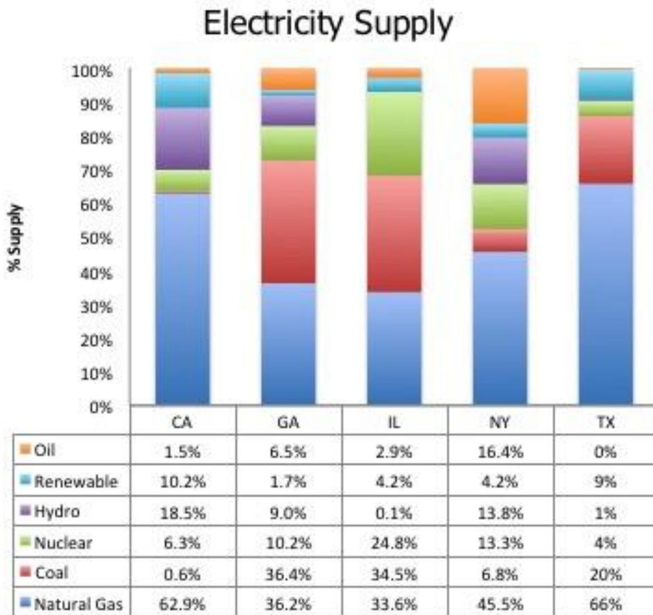
Figure 3.15 Differences in regional electricity generation supply
