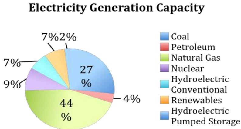
Figure 3.5 Electricity generation capacities by type
