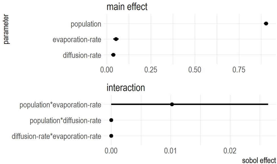
Figure 4: Main effects (upper panel) and interaction effects (lower panel) of each parameter of the Ants model on the total number of simulation steps that were simulated until all food sources were depleted by the ant individuals. Parameter effects were derived by applying a Sobol sensitivity analysis approach. Points indicate parameter mean sensitivity (Sobol effect) of 6 model simulation replicates, linebars indicate the corresponding standard deviation.
