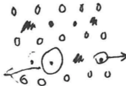
Figure 11: Kim’s sketch of the lattice. Open circles are iron atoms and filled in circles are carbon atoms. The two circled carbon atoms with arrows are her indication of how they might diffuse.
