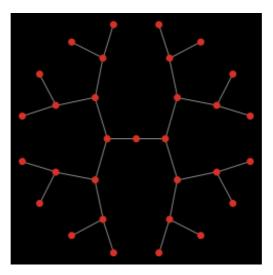
Given a set of anchor nodes <u>layout-tutte</u> places all the other nodes at the center of mass of the nodes it is linked to. The anchor set is automatically arranged in a circle layout with a user defined radius and the other nodes will converge into place (this of course means that you may have to run it several times before the layout is stable.)
