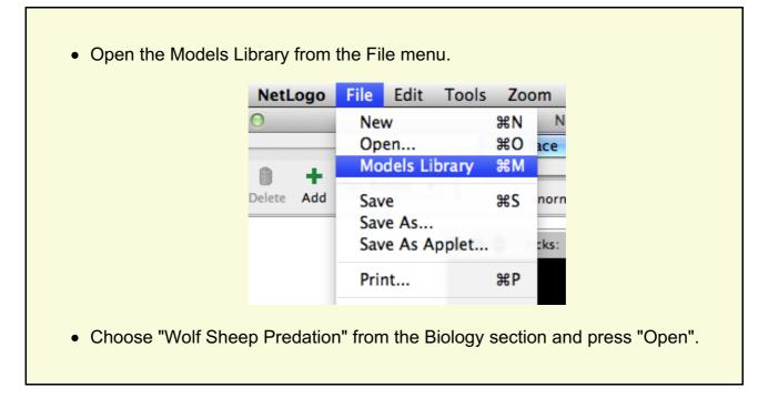
The Interface tab will fill up with lots of buttons, switches, sliders and monitors. These interface elements allow you to interact with the model. Buttons are blue; they set up, start, and stop the model. Sliders and switches are green; they alter model settings. Monitors and plots are beige; they display data.
