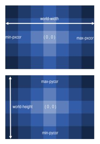
In these diagrams, max-pxcor is 3, min-pxcor is -3, max-pycor is 2 and min-pycor is -2.
