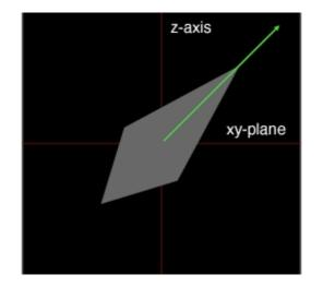
Roll is the rotation around the turtle's forward vector. It is relative to heading and pitch.
