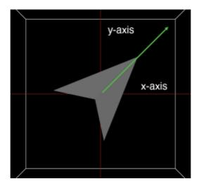
Pitch is the angle between the nose of the turtle and the xy-plane. It is relative to heading.
