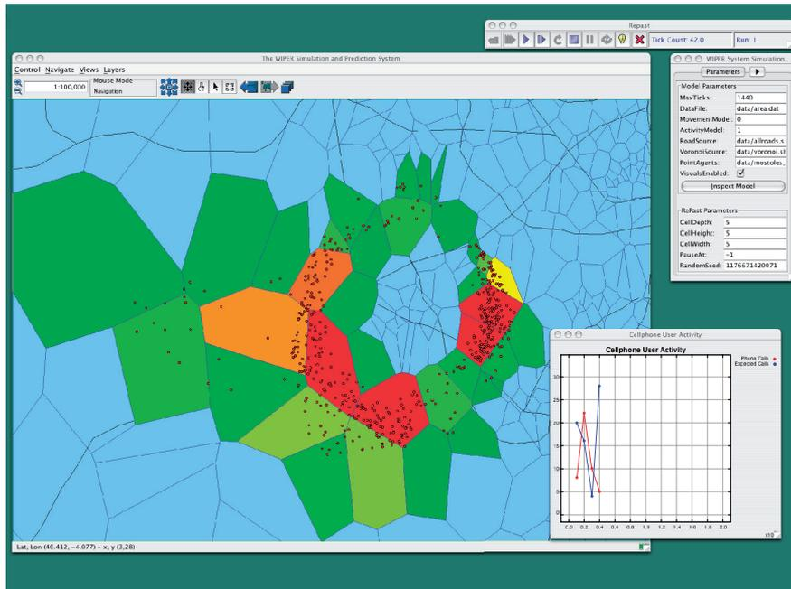
Figure 3. Screen shot of the wiper simulation. This simulation is a flee movement model with distribution-based activity model. Agents are represented as red dots with the voronoi cells colored by the number of agents.
