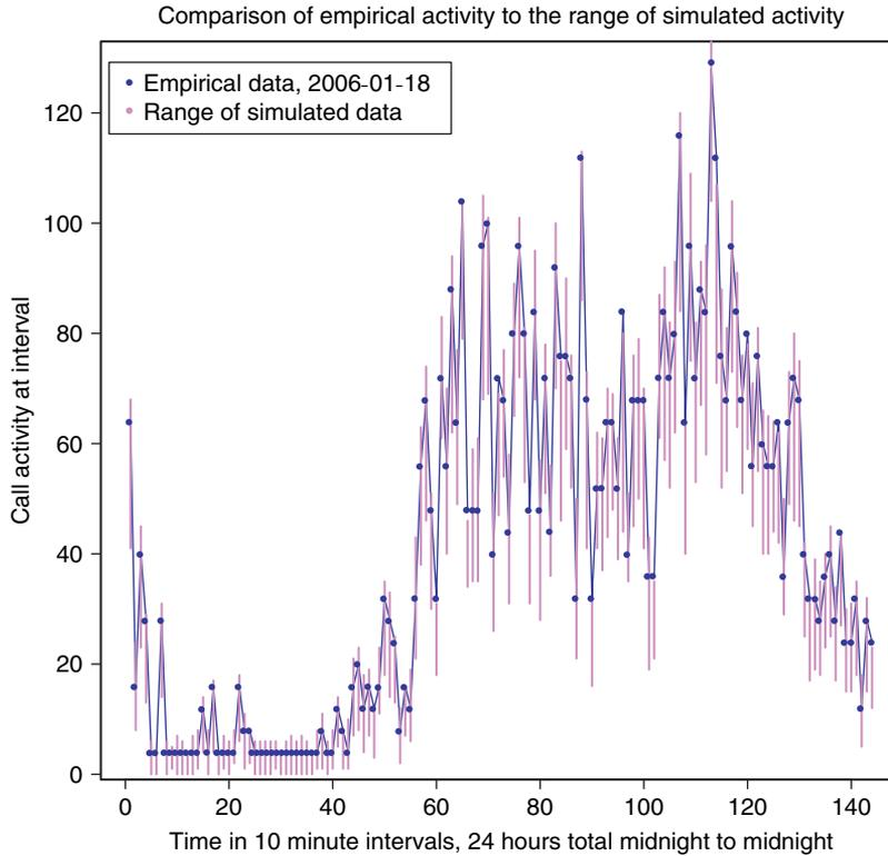
Figure 1. Plot of empirical call activity over the range of simulated call activity, demonstrating that the simulation generates activity without bias.
