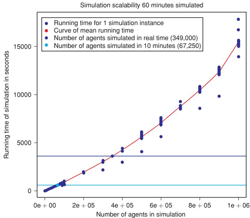
Figure 4. Simulation scalability with respect to number of agents, 20 replications at each level. In this instance we run simulations for 60 minutes of simulated time. In this graph we examine agent simulations out to a population size of 1,000,000 agents.
