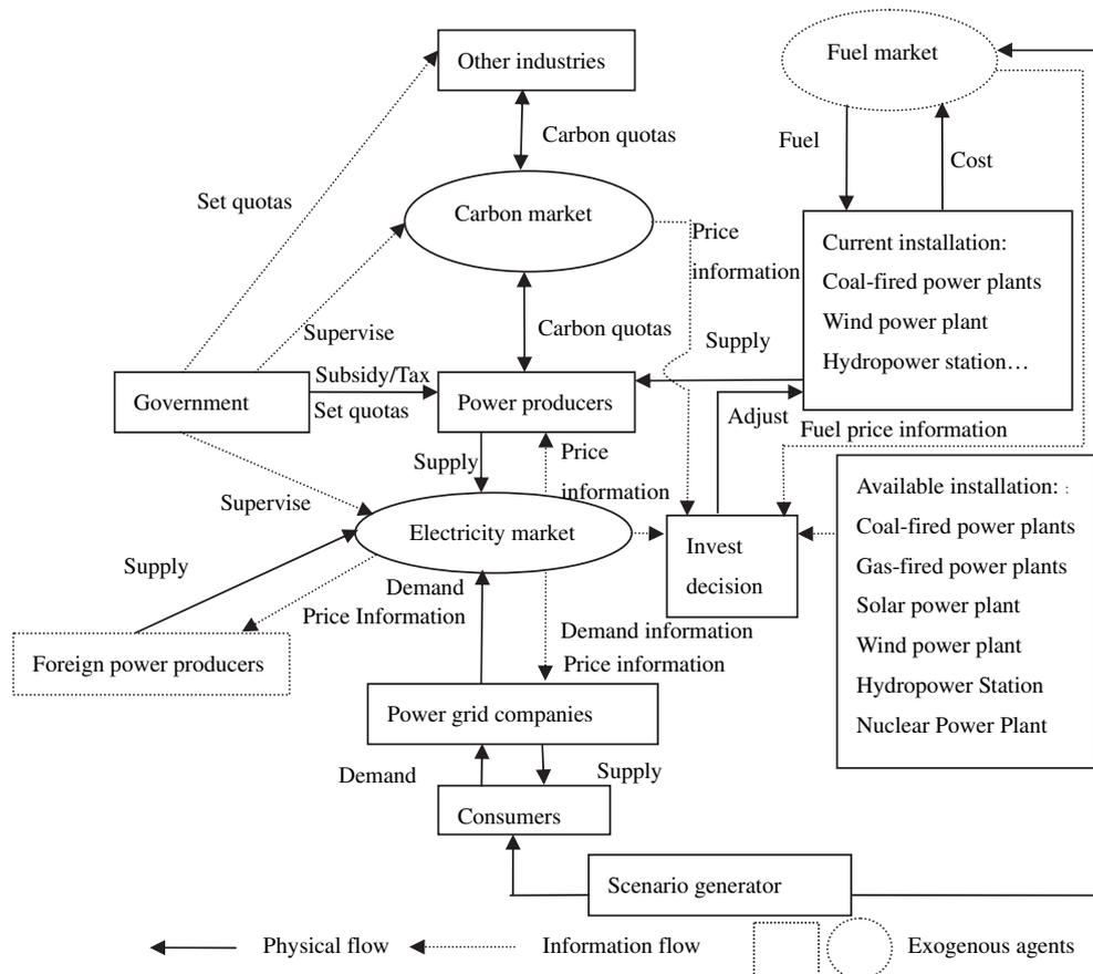
Fig. 1. System structure.
