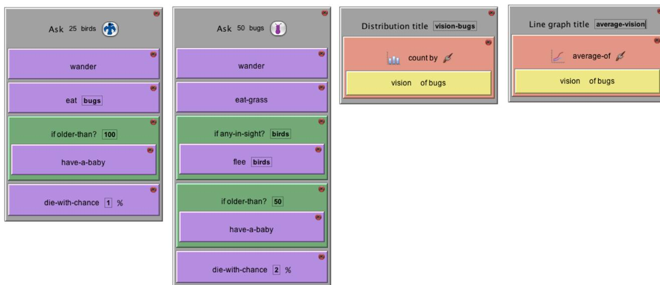
**Fig. 1** Code for a model representing two species, birds and bugs, and their respective rules. The model also includes two plots, a histogram tracking vision range of bugs and a line graph tracking the average vision range of bugs
