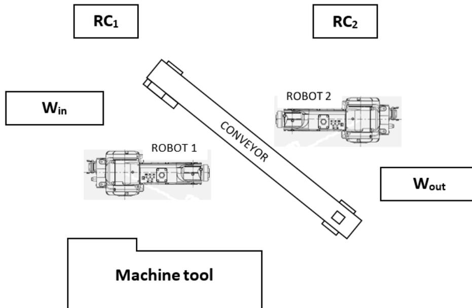
**Figure1.** Model of a robotized production workcell.
