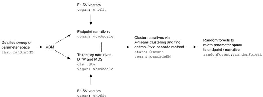
**Fig. 2** The analysis tool chain used to identify narratives. Text in courier font refers to R (R-Development-Core-Team 2016) packages and commands. SV = state variable
