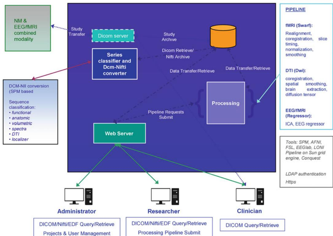
**Fig. 4** Operative scenario of the integrated framework
