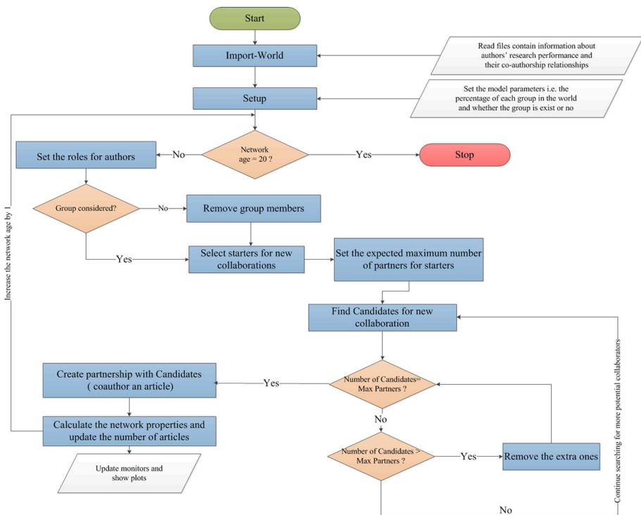
**Fig. 1** Flowchart of the developed simulation model
