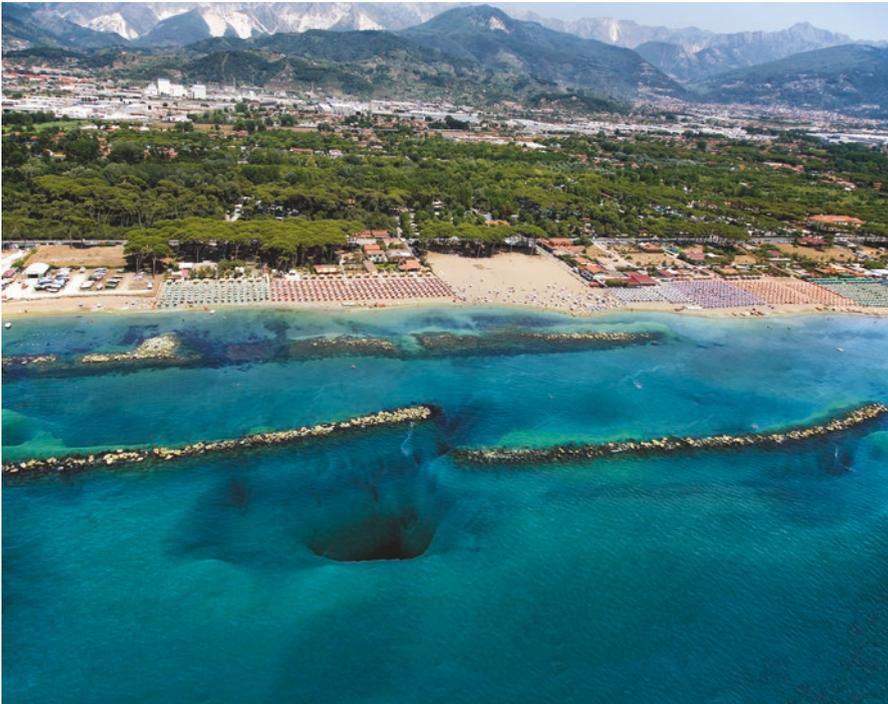
**Fig. 20.5** Deep hole at the gap of detached breakwater excavated by offshore currents induced by piling-up (vertical exaggeration; Geocoste s.r.l.)
