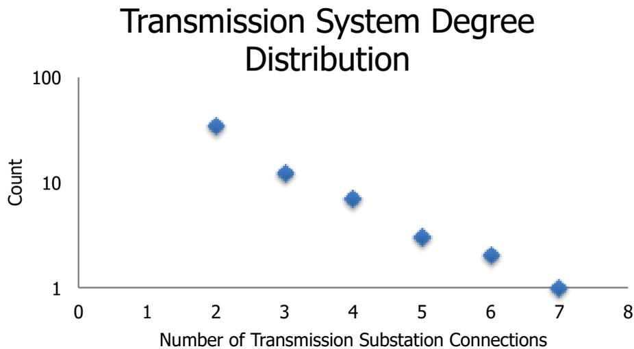
Figure 3.6 Connectivity of transmission grid is scale free
