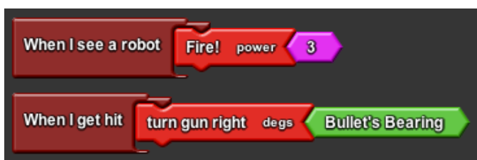
Figure 9. The two main methods of Beth's strategy after discovering the Bullet's Bearing block.
